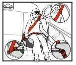
Place the child into the booster seat, and fasten him/her with the vehicle 3-point passenger seat belt. The upper part of the diagonal strap must rest on the child's shoulder. The lower part of the diagonal strap must be over the armrest, with the lap belt running under both armrests of the booster seat.
