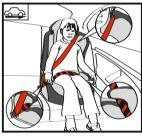
• Place the child into the child car seat, and fasten him/her with a vehicle 3-point passenger seat belt. The upper part of the diagonal strap must rest on the child's shoulder. The lower part of the diagonal strap must be over the armrest, with the lap belt running under both armrests of the child car seat.
