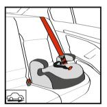
• Place the booster seat on the vehicle seat facing forward.
