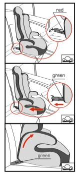
Place the child car seat on the vehicle seat, positioning the locking arms right in front of the ISOFIX anchorage points (insertion aids).
