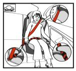
• Place the child into the child car seat, and fasten him/her with a vehicle 3-point passenger seat belt. The upper part of the diagonal strap must rest on the child's shoulder. The lower part of the diagonal strap must be over the armrest, with the lap belt running under both armrests of the booster seat.
