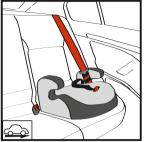
Place the booster seat on the vehicle seat facing forward.
